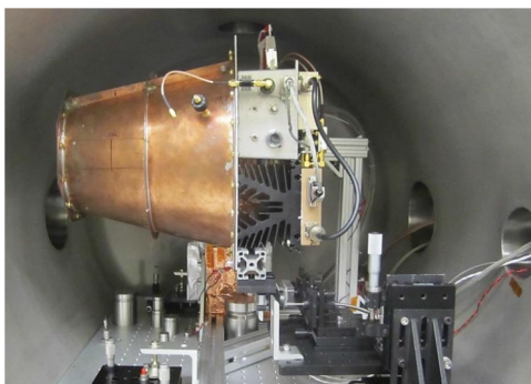
Fig. 14 Forward thrust mounting configuration (heat sink is black finned item between test article and amplifier).
